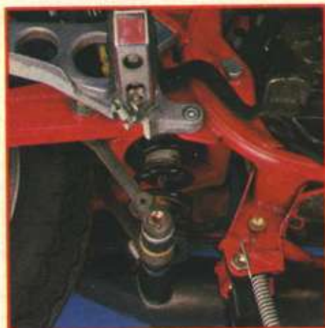
Mono-X shock absorber mounts low The RZ's link to the TZ-world.
