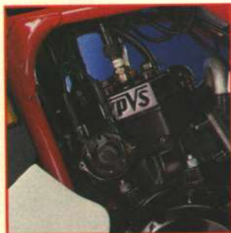
Power Valve cable mechanism Pushing and pulling for more power.
